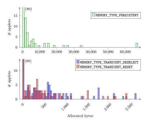
Fig. 11. Histograms of memory allocation in entry point class constructors per applet on NXP JCOP4 J3R180 with maximum available transient memory around 3.8 kB. Note that the first largest bin is clipped in both graphs.
