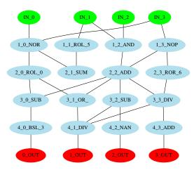
Fig. 1: Software circuit with input nodes  $(IN_x)$ , inner nodes, output nodes  $(x_OUT)$  and connectors. Note that not all input or output nodes need to be used as well not all inner nodes need to output any value.
