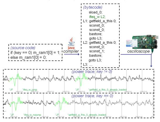
Figure 4: Example of process of reverse engineering of Java Card applet. By tecode instructions are visible in power trace and allow to distinguish whether then or else branch was taken based only on  $if_{-eq}$  operation.
