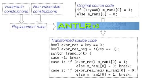
Figure 5: Automatic replacement framework process. Templates of vulnerable constructions and their secure secure replacement are combined in the replacement rules. ANTLR parser is used to automatically transform source code of the applet.
